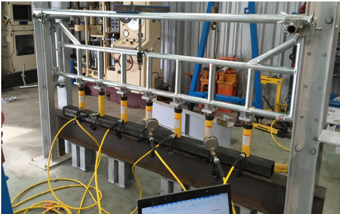
Typical image of Load Bay Beam test assembly
