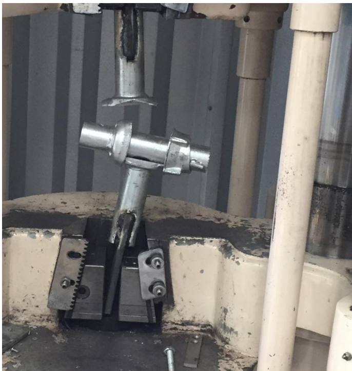
Post load image showing separation. Blade and cup yield evident, blade tip Distortion and cup distortion evident.
